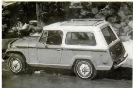
JEEPSTER COMMANDO has some ruggedness and 4wd as Universal, can be made as wagon, roadster or pickup; uses same F-head 4 or V6 as regular Jeep
